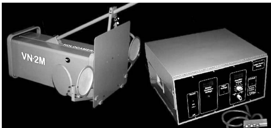
Equipment needed for single-shot holograms of extended objects
