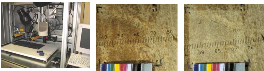
Figure 4: Workstation for laser cleaning of paper. An example is reported.
