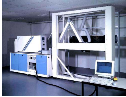
Figure 3: Laser workstation for cleaning of painting
